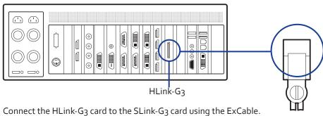
(ExCable-G<sub>3</sub>, packaged and shipped with the expansion unit).
