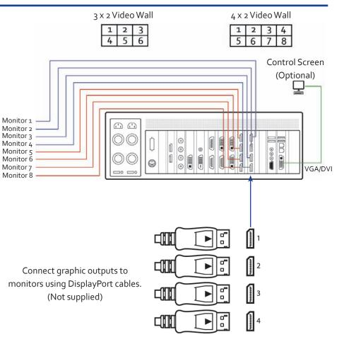
Many of our wall controllers are configured to use a control screen prior to leaving the factory, if required, connect the control screen to the SBC as shown above. If a control screen is not required, the BIOS settings will require changing, see User Guide for detailed instructions.
