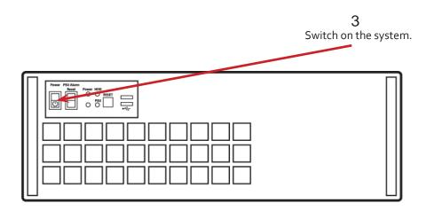
If you have an VSN Expansion Chassis connected to the main unit then the power supply units on the expansion chassis should be switched on prior the main unit. There is no requirement to "switch on the system" (3) on an expansion chassis.
